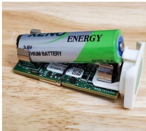
Figure 2-6: Battery Polarity Orientation
