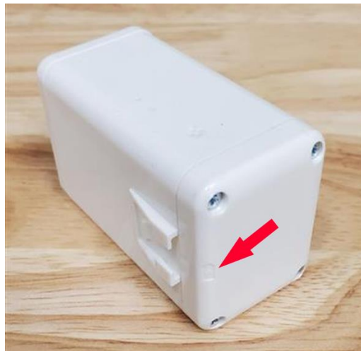
Figure 2-11: Proper Replacement Orientation of the Battery Cover
