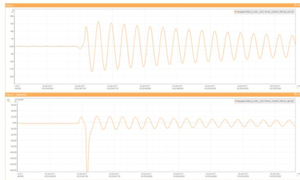
Figure 6: Fault record example  $U_o$  and  $I_o$
