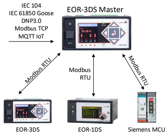
For switch gears, where a motor control unit (MCU) is installed for switching of circuit breakers, this way it is possible to connect MCU units via Modbus.
