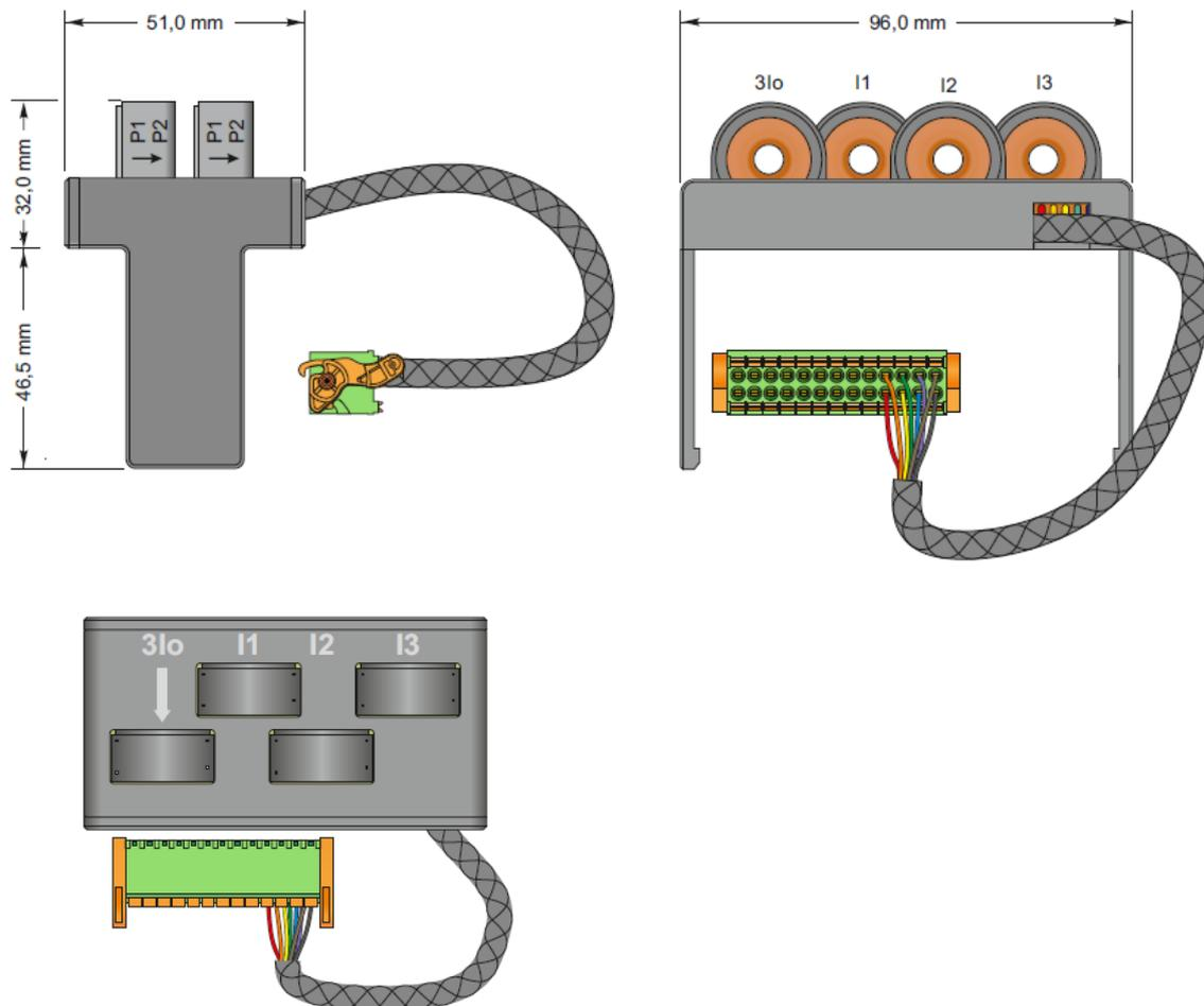
Figure 17: Dimensions of plug-on adapter for classical current measurement feature C21
