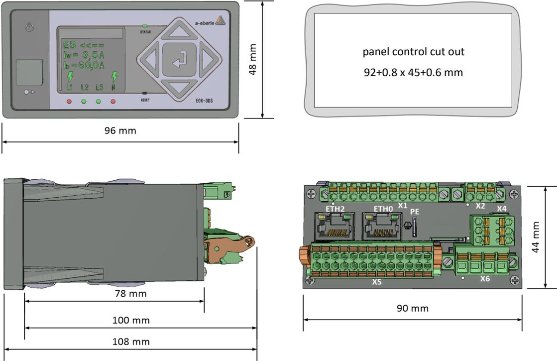
Figure 15: Dimensions EOR-3DS with feature U05/U06/U07 with C10
