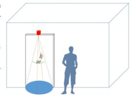
SenlabP logs the number of passage and allows 2 functional modes (see Understand the two SenlabP functional modes section for more details):
