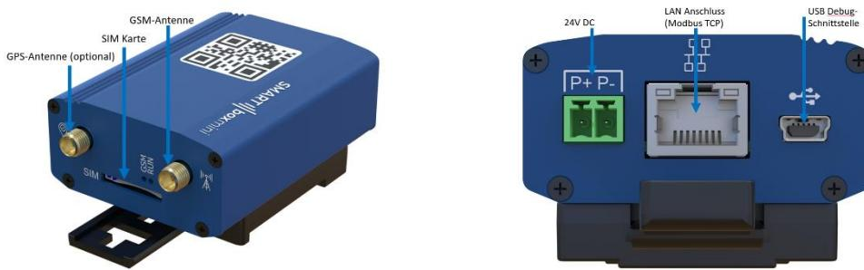
◊ The ramp-up of the unit takes about 60. When the "IOT and Run" LEDs flash, the unit is ready for use. Searching for the mobile network can take up to 15 minutes. If the IoT LED is still in the status of continuous lighting, either the SIM card is not activated, not engaged correctly or an external antenna must be used.
