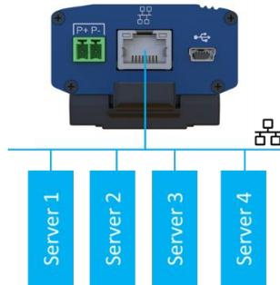
Specification A Modbus TCP client connection is available at the gateway with connection of max. 4 servers. Attention: When connecting directly to the server without a switch, a cross cable must be used
